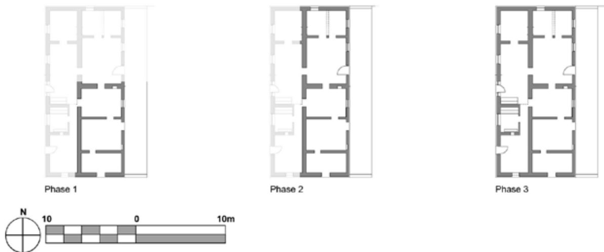
Figure 5 Measured plans of House Venter on Modderfontein near Fouriesburg indicating the original house and the two phases of additions, from linear house to double bank house (plans measured and drawn by the author).
