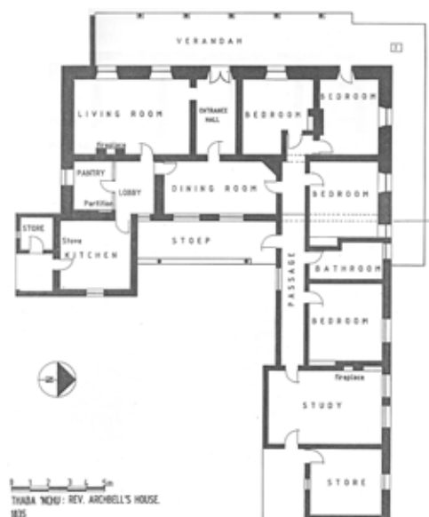
Figure 3 Measured plan of the Reverend Archbell's House of 1835. Original house with thick walls to the top with later additions in thinner walls to the bottom (source: Roodt 1987, plate 2).
